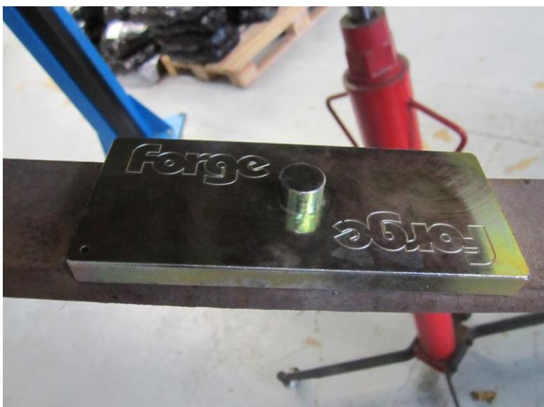
9. With the offset plate in the correct position lift the leaf spring back into place ensuring the pin locates inside the hole. Refit the bolt at the rear of the leaf spring as seen in step 4.
