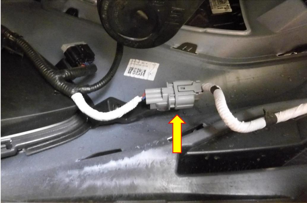
7. Unplug both the temperature sensor and the AAC sensor.
