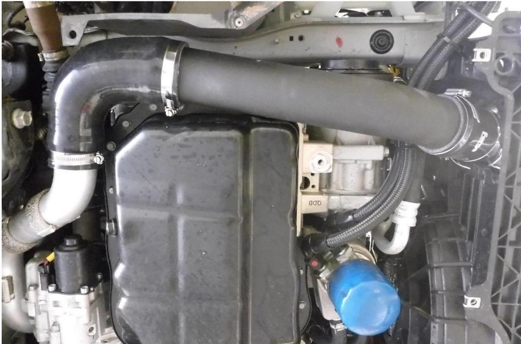
17. Now fit the near-side hose to the intercooler. This is also secured with 7mm hose clamps, the same as the off-side hoses.
