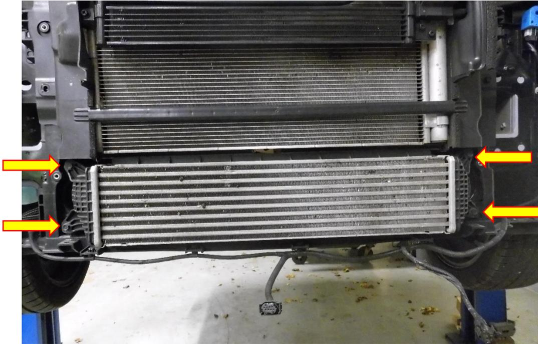
12. The rest of the off-side intercooler hose can be taken off the car, loosen the 8mm hose clamp in the same way as before, then undo the fastener holding the OE hard pipe to the car with a 10mm socket and ratchet drive. Now remove the hose and pipe as one, from the vehicle.
