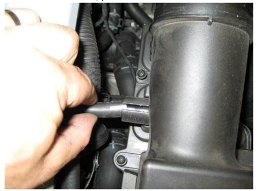
3. Undo the 5mm allen bolt that holds the airbox in place
