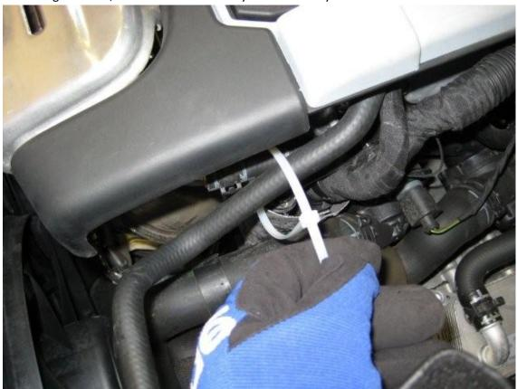
10. Attach the ducting to the end of the carbon fibre airfilter box NOTE the orientation of the box – the inlet and outlet have arrows above them showing the direction of air travel (in and out).
