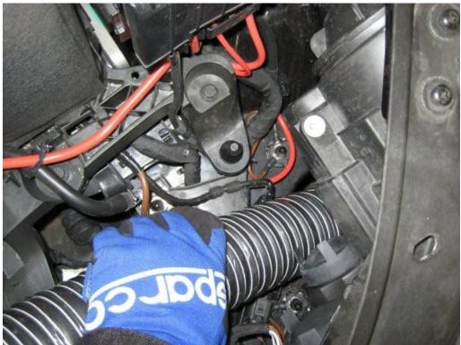
....and push the airfilter box into the silicon joiner
