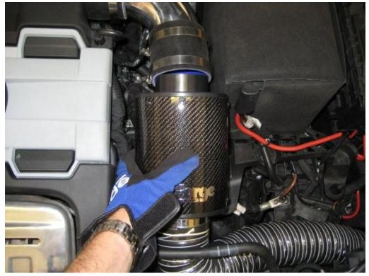
12. With the clips still loose, you should be able to rotate the whole airbox assembly up and down so that it doesnt hit the underside of the bonnet, or the pipes under the filter. When you are happy, tighten all the jubilee clips.
