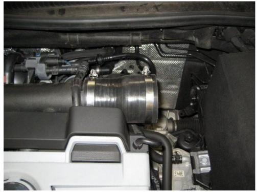
8. Insert the 90 degree aluminium bend into the end of the reducer, and connect the small bore 8mm pipe that came from the side of the airbox into the barb on the underside of the bend, then put the Forge straight silicon coupler on the end of the aluminium bend, together with two 70-90mm jubilee clips (again dont tighten).
